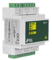
The MIO 24 unit is a process signal concentrator that uses RS-485 communication and allows for remote signal display. Likewise, the MIO 24 unit has 4 analogue inputs that operate in the 0 to 20 mA range. The unit handles standard proportional industrial measurement signals and operates in linear form throughout the input range.
