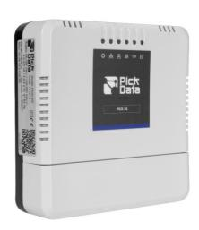
Pick 3G is a gateway designed to communicate with machines and sensors, collect and store their data and send it to the website for their treatment.
