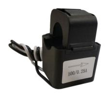
**TRA1 100A transformers** are current transformers specially designed for being installed at the top of a circuit breaker. All the models have secondary of 250 mA and are suitable for SEM One, SEM Three and third-party devices.
