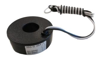
**TRC1 250A transformers** are current transformers specially designed for being installed at the top of a circuit breaker. All the models have secondary of 250 mA and are suitable for SEM One, SEM Three and for third-party devices.
